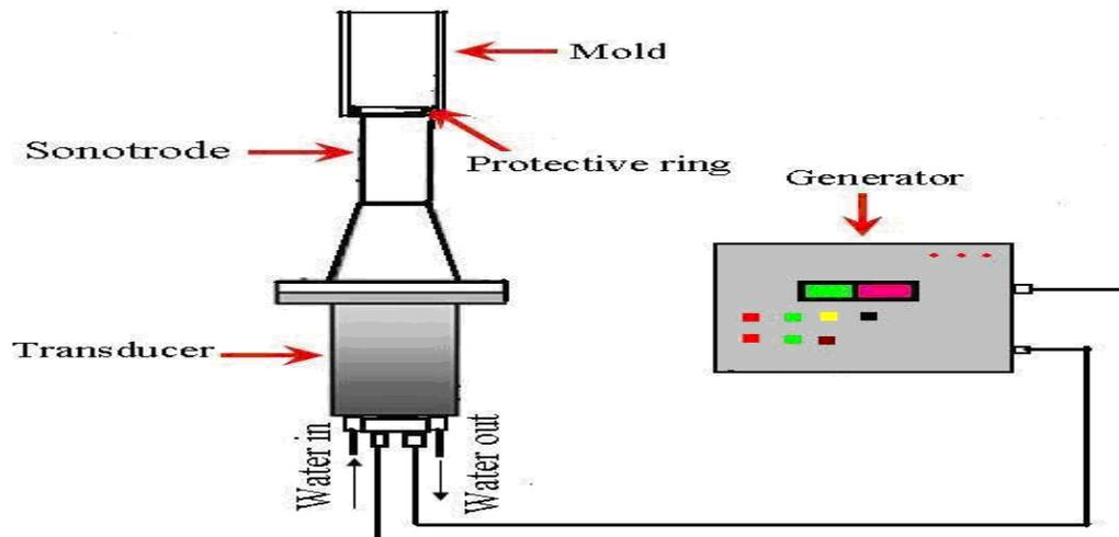
Fig.1 The setup experiment of ultrasonic treatment equipment.
