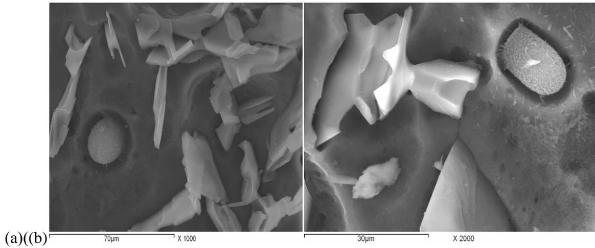
Fig. 5 SEM photomicrographs identification of intermetallic phases  $\alpha$ -Al<sub>15</sub>(Mn,Fe)<sub>3</sub>Si<sub>2</sub>,  $\beta$ -Al<sub>5</sub>FeSi and  $\delta$ -Al<sub>4</sub>FeSi<sub>2</sub> of the as-cast A356 with ultrasonic vibration at different magnification (a&b)
