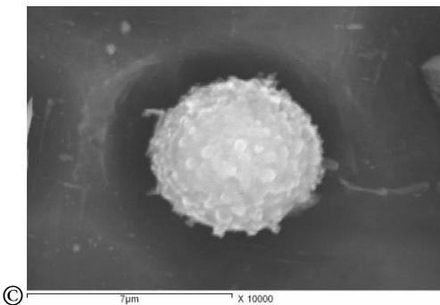
Fig. 6 SEM photomicrographs identification of intermetallic phases  $\alpha$ -Al<sub>15</sub>(Mn,Fe)<sub>3</sub>Si<sub>2</sub>,  $\beta$ -Al<sub>5</sub>FeSi and  $\delta$ -Al<sub>4</sub>FeSi<sub>2</sub> of the as-cast A356 (b) without ultrasonic vibration. (a& c) with ultrasonic vibration at different magnification.
