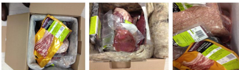
Figure 2. Sample boxes with meat (left-right: Wool lined, Wool unlined, expanded polystyrene).
