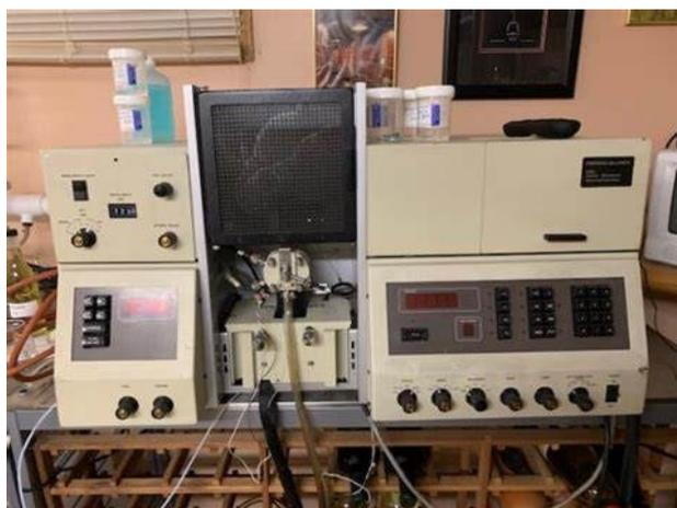
**Figure: (2)** The Atomic Absorption Spectrophotometer (AAS)
