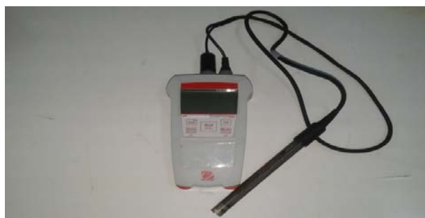
Figure: (3). The PH device used to measure acidity in the Henna samples.
