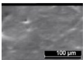
Figure (4): SEM image of charred PP-NOR-107 heated sample.
